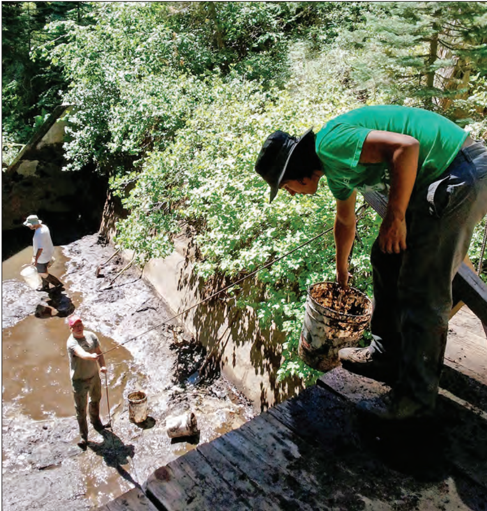
Figure 6—Sediment is removed, weighed, and sampled to quantify and characterize the annual load in a stream. A sediment basin is emptied at the Teakettle Creek, which is used as a control watershed in the Kings River Experimental Watersheds.
