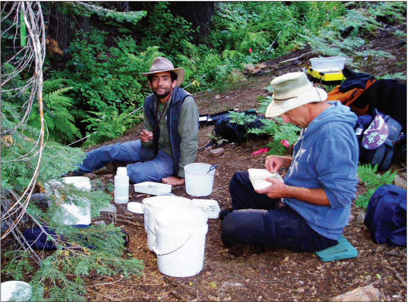
Figure 7—Benthic macroinvertebrates are collected from streams with nets, woody material is removed, and organisms are sorted in the field before being preserved and taken back to the laboratory for identification.
