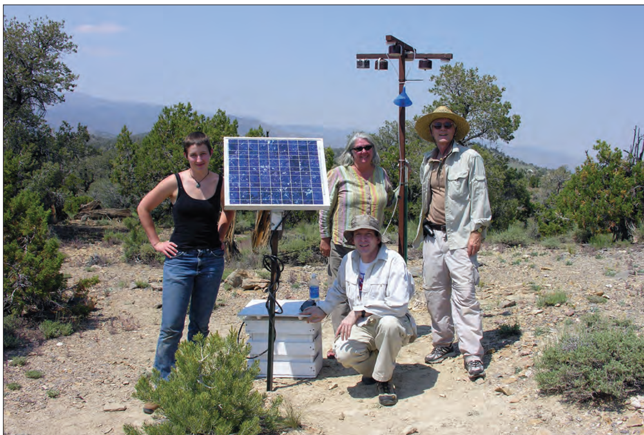
Figure 2—Air pollution monitoring site with active ozone instrument and passive samplers in the White Mountains of California during 2007. Research was conducted by collaborators from the USDA Forest Service Pacific Southwest Research Station, University of California, and Saint Mary’s College.
